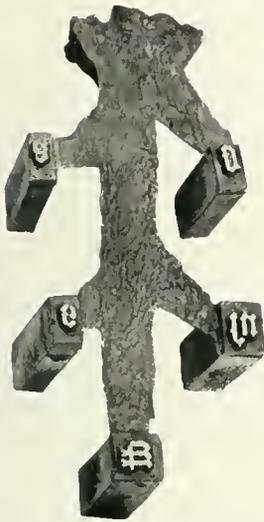
FIG. 1. SPRAY OF LEADEN TYPES CAST IN SAND IN A TWO-PART BOX.
