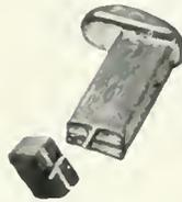
FIG. 3. SAME TYPE BROKEN SHOWING IMPRESSION OF NICK.
